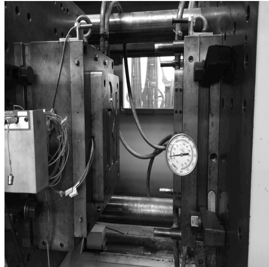
Figure 2: ASTM mold in a Sumitomo 180 Ton injection-molding machine
